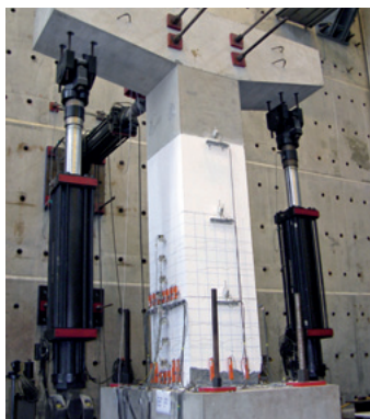
Fig.2 Segmental pre-cast bridge column system possessing high energy-dissipation capability and low residual displacement
