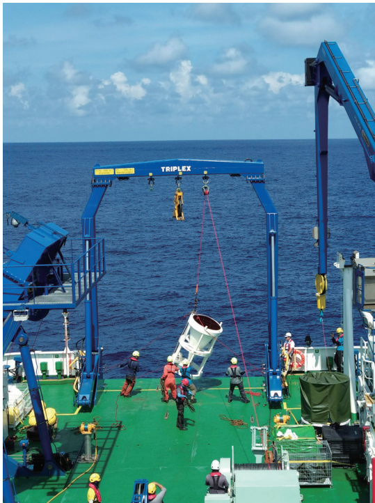
Deploying the mooring system of sediment trap
