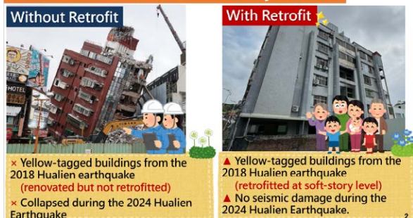
▲ Effectiveness of seismic soft-story retrofitting.
