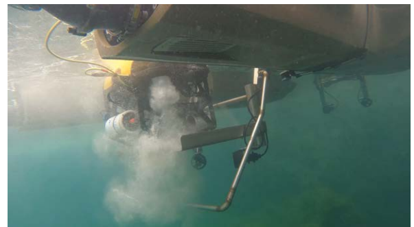
▲ Remote control of a surface unmanned vessel to deploy an observational ROV.
