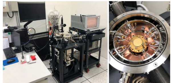
▲ Chip-level testing platform capable of reaching -269^{\circ}\text{C} .
