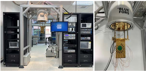
▲ Circuit-board-level testing platform capable of reaching -269^{\circ}\text{C} .
