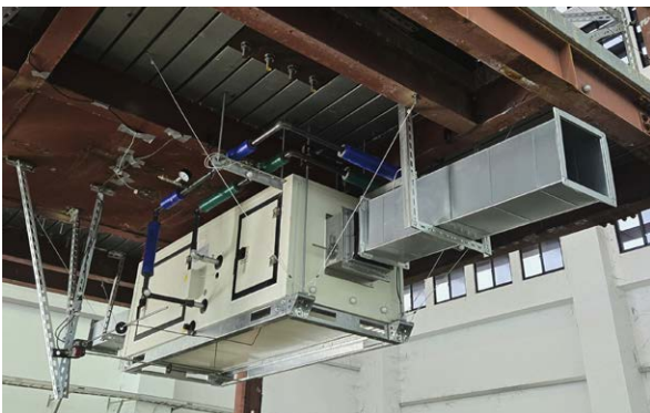
◀ Test specimen of a suspended air conditioning unit.
