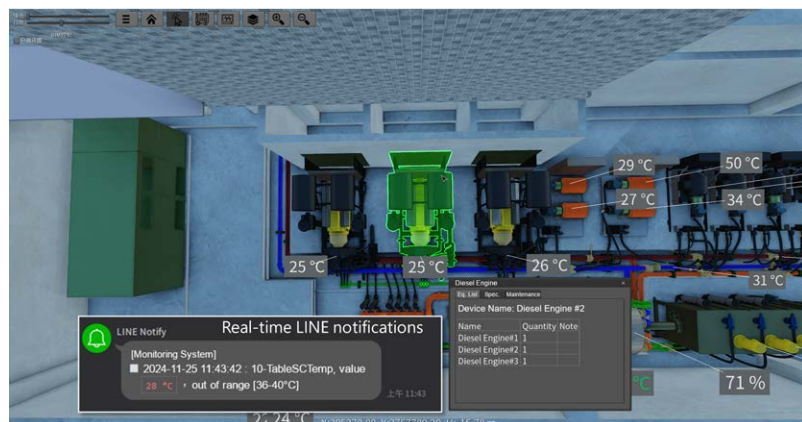
◀ Real-time LINE notifications of abnormal conditions and data monitoring.
